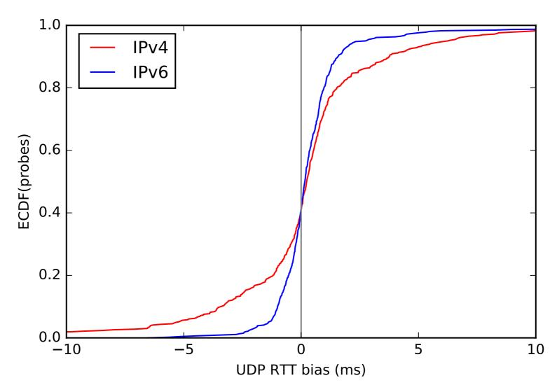
Median RTT bias, UDP/33435 vs TCP/33435, 464 probes to APNIC anchor Feburary 2016
