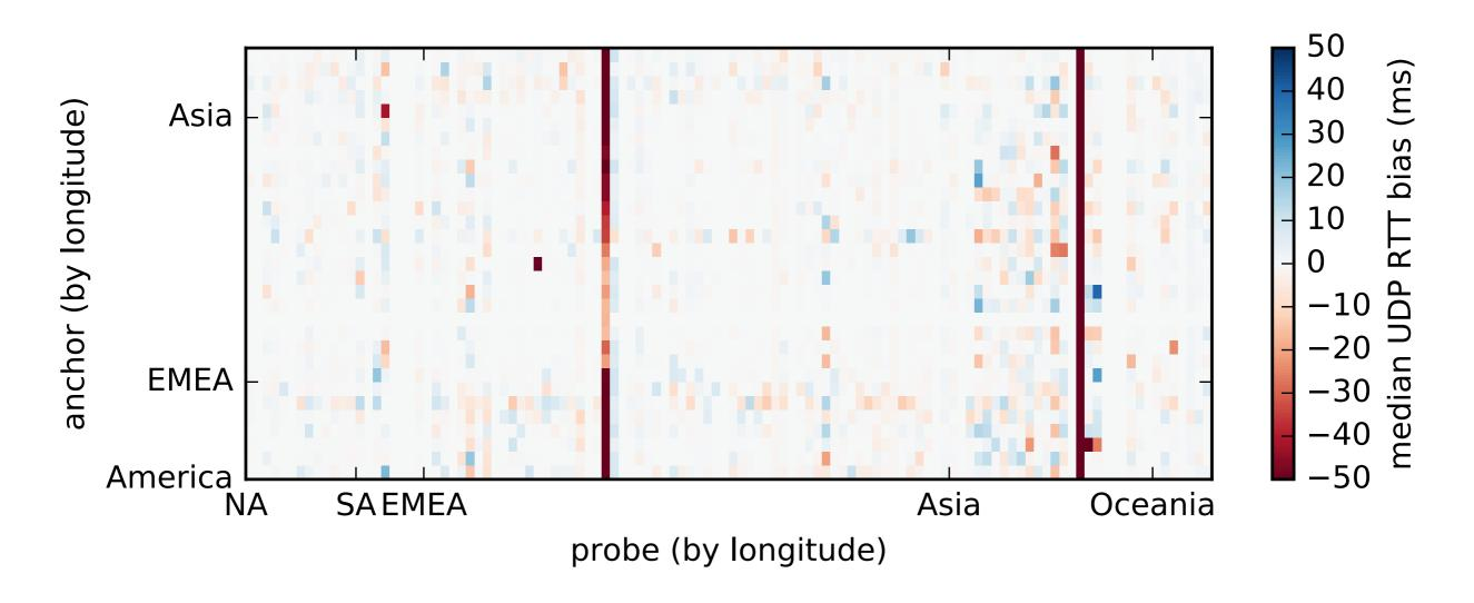
Median RTT bias, UDP/33435 vs TCP/33435, <= 19 trials, 128 probes to 32 anchors September 2015
