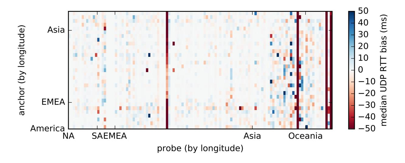
Median RTT bias, UDP/33435 vs TCP/80, <= 19 trials, 128 probes to 32 anchors September 2015
